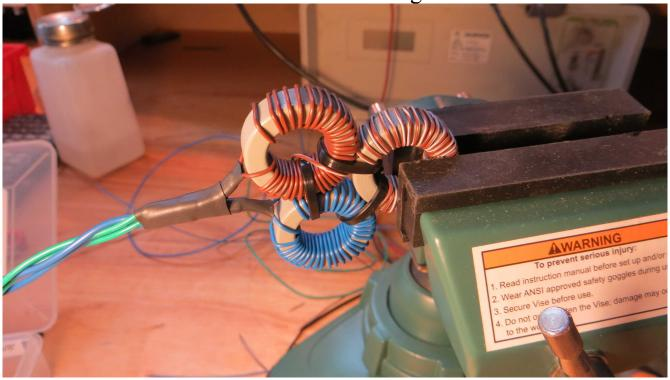
Just strip and tin opposite ends and that is it. Your primary line will go through the center of the first ferrite core. The one at the tip of your triangle. (The one being clamped in the picture.)
